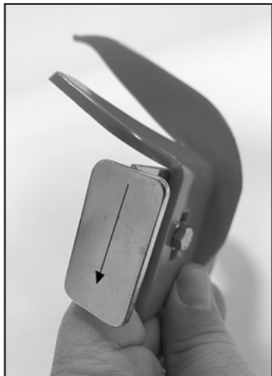
Detail of peeler shaft assembly
